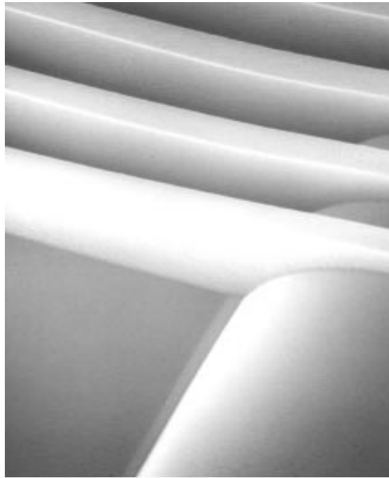
Figure 11: Multilayer Resist ( 2\ \mu\text{m} lines in 10\ \mu\text{m} of resist over 6\ \mu\text{m} structures)
