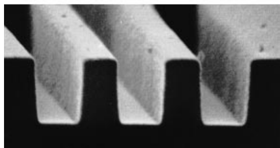
Figure 15: Cross section views of 0.6 and 0.7 micron lines and spaces patterned on the 2244i
